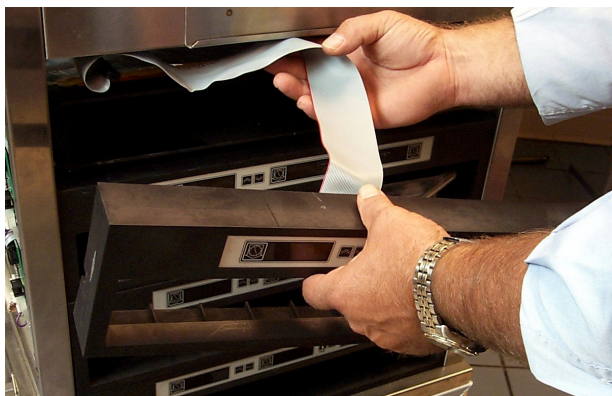
Fig: 3 Feed ribbon cable out of UHC when bezel is removed.
